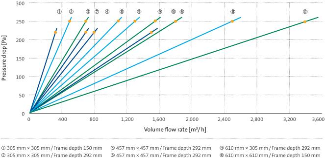
③ 305 mm × 305 mm / Frame depth 292 mm 457 mm × 457 mm / Frame depth 150 mm
