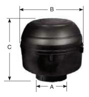
To properly size a Fleetguard Pre-Cleaner, you will need to know the correct airflow of the engine in CFM (m³/min) and the Outside Diameter (OD) of the air intake. For optimum efficiency, select the pre-cleaner where the CFM (m³/min) falls in the upper end of the ranges shown. **Do not size a Fleetguard Pre-Cleaner solely based on the air intake dimension.**
